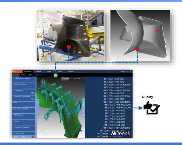
Accurate Registration of NC into the 3D Database, Providing Quick Access to Information for Disposition
