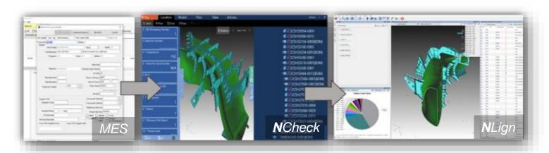
Accurate Registration of NC into the 3D Database, Providing Quick Access to Information for Disposition
