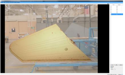
These images show the damage to the mapping process. First, a photograph is taken of the damage. Next, the photograph is aligned with a CAD model. Finally, the damage in the photograph is mapped onto the CAD model
